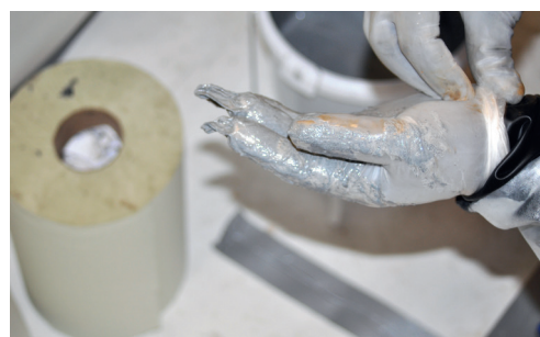
4. The glove is removed by grasping the wrist of the glove.
