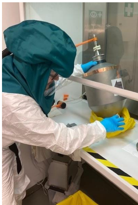
A dust drum containing graphene powder is emptied and cleaned in a fume hood. The worker is using a filter protector (TH3P) with a fan and a hood, type 5 protective clothing and nitrile gloves.
